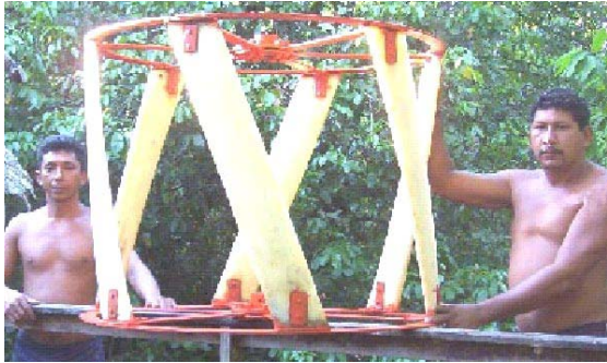
Figure 2. 6-blade Gorlov turbine used in rural Amazon electrification project
