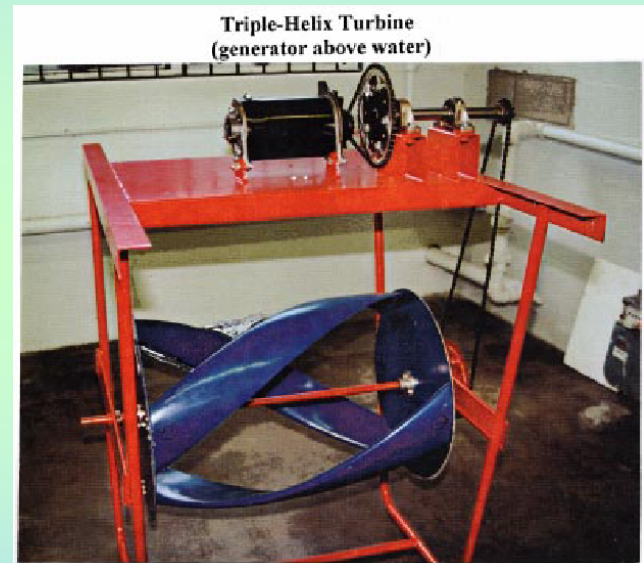
3 blade Gorlov turbine with electric generator to be connected to BioRock structure
