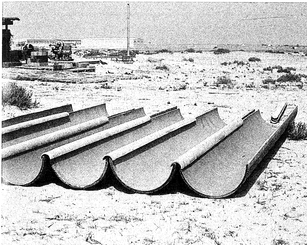
Examples of research on fiber-cement roofs and walls undertaken for the United Nations Centre for Human Settlements by the author of this article. The basic concepts are still relevant for use with the results of mineral accretion of seawater, in order to obtain strength by shaping the building components. Generally the cost of roofing represents up to 30 per cent of the entire expense of basic low-cost house. Therefore, research towards reducing roofing costs is highly important.
