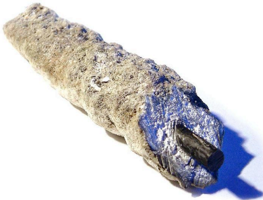
Two years of Biorock material growing on iron bar. Photo Wolf Hilbertz.
