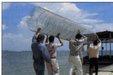
6. Light mesh cathode for fabrication of roofing components before submersion. Photo: W.H. Hilbertz.
