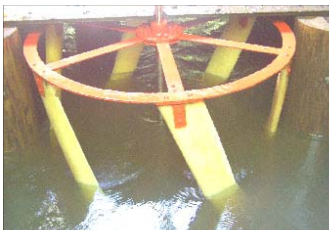
6-blade Gorlov Helical Turbine
