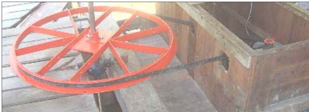
Pulley, 1.08 m (43 in) in diameter, and belt
