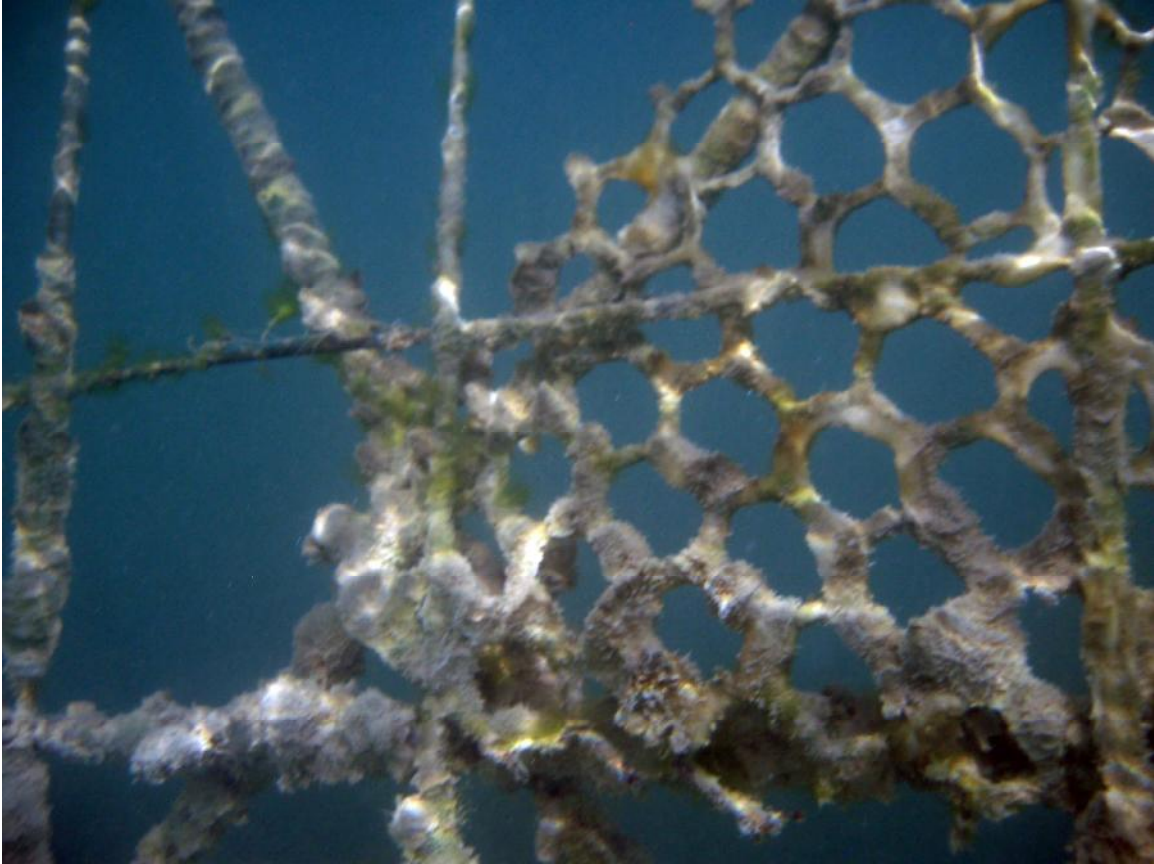
Figure 10. After just two days of wind power limestone minerals are growing over the reinforcing bars and wire mesh.
