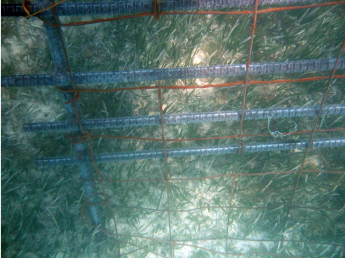
Figure 14. One day after connection to the wave generator, the rust has completely disappeared from the steel bar and they are turning white with new limestone mineral growth. The thinner mesh draws less power and is still rusted, but the rust is starting to reform and will also vanish in a few days.
