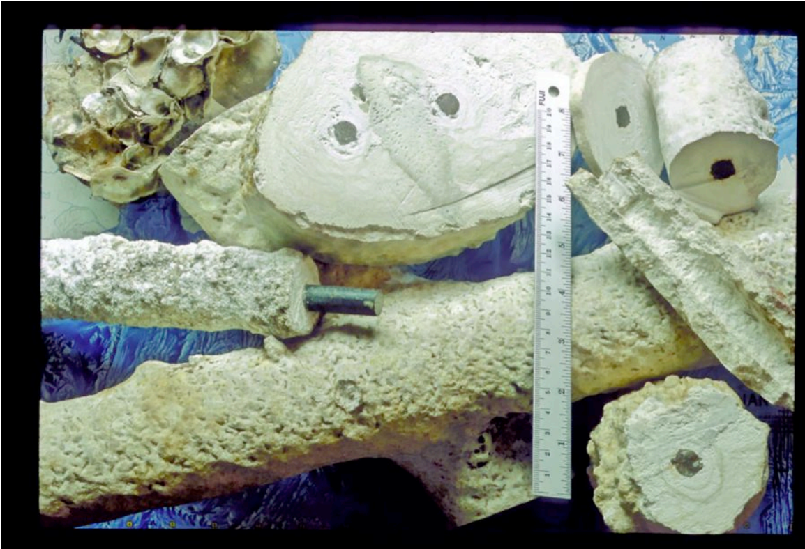
Various pieces of Biorock cut out of structures, showing un-rusted original steel inside, covered with limestone rock grown over them. Photo Wolf Hilbertz.
