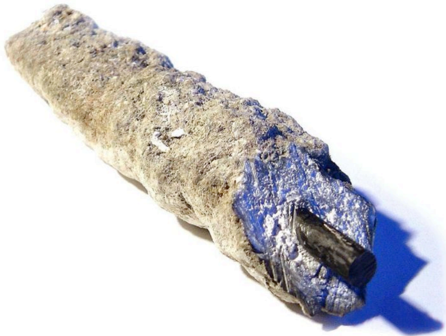
Two years of Biorock material growing on iron bar. Photo Wolf Hilbertz.
