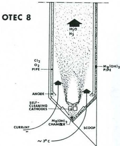
Fig. 31. Functions of proposed OTEC plant.
