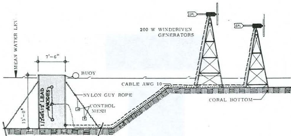
Fig. 25. Circular column and wind driven generators.
