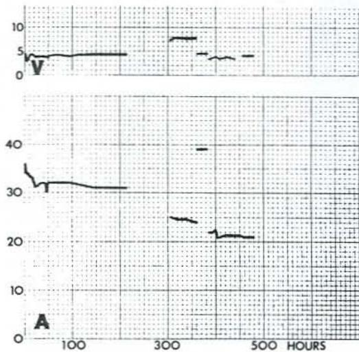
Fig. 13. Consumption of electricity, artificial Reef 1.
