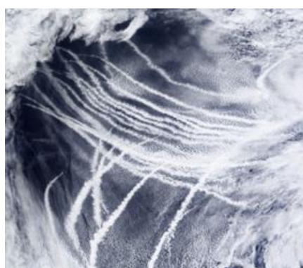
Figure 14 Satellite image of cloud formation generated by ship exhausts
