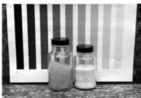
Figure 13 Demonstration of Twomey effect with 4mm and 40 micron glass balls (courtesy of Stephen Salter)
