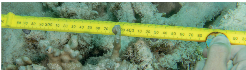
Figure 2: As a reference for the original size of the natural reef, we took about 25 manual measurements to scale both reconstructed 3-D point cloud models and to calculate deviations between the original and digital reconstructed 3-D model.
